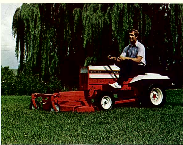
Gravely 814, 14 HP Riding Tractor with 50-inch Front-Mount Rotary Mower, Front Drive Kit
