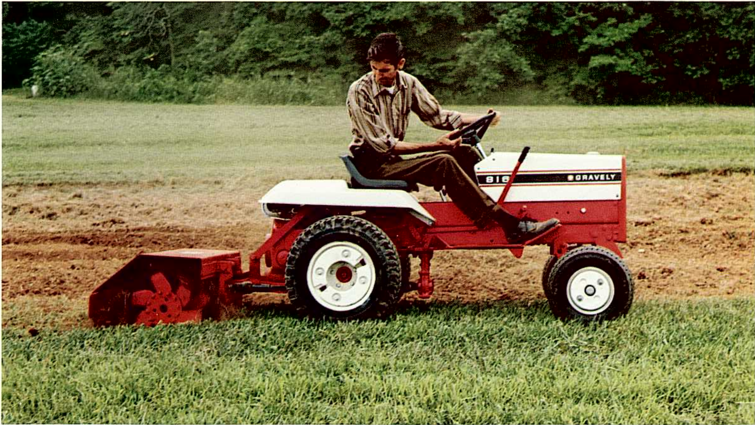
Gravelly 816, 16.5 HP Riding Tractor with Rear Tiller, Rear P.T.O. Kit, and Wheel Weights
